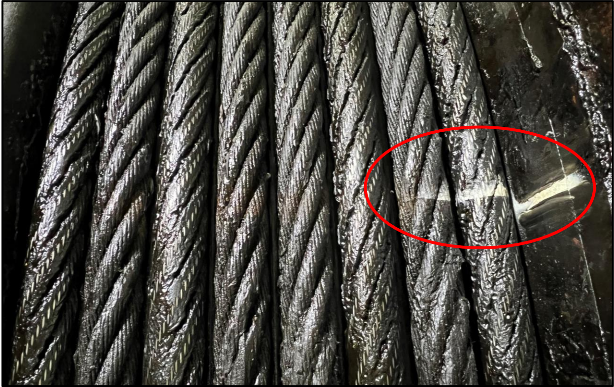
Photo 1: White Markings on the Wire Rope and Sheaves Indicating Rope Slippage
