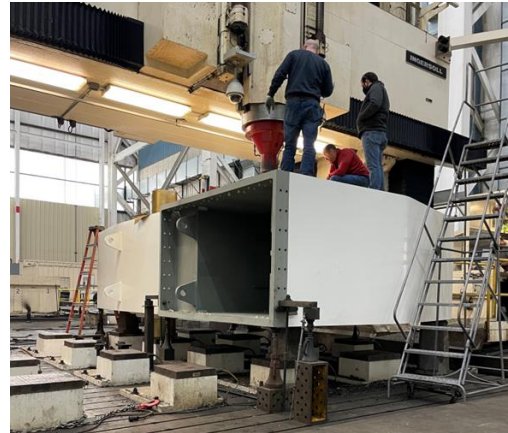
Machining a counterweight girder
