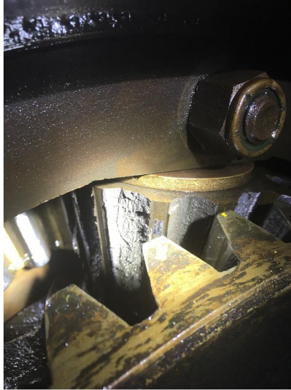
Figure 2: East Gear Reducer, Broken Gear
