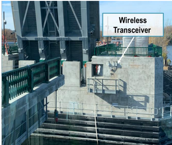
PHOTO 15: Wireless Transceiver Mounted On Pier Wall
