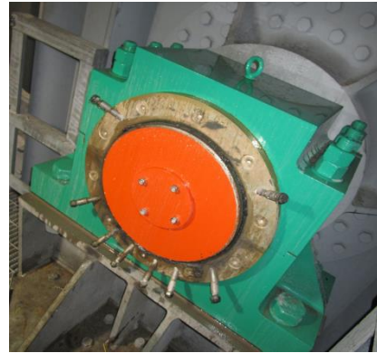
PHOTO 9: Painted Trunnion Bearing Assembly
