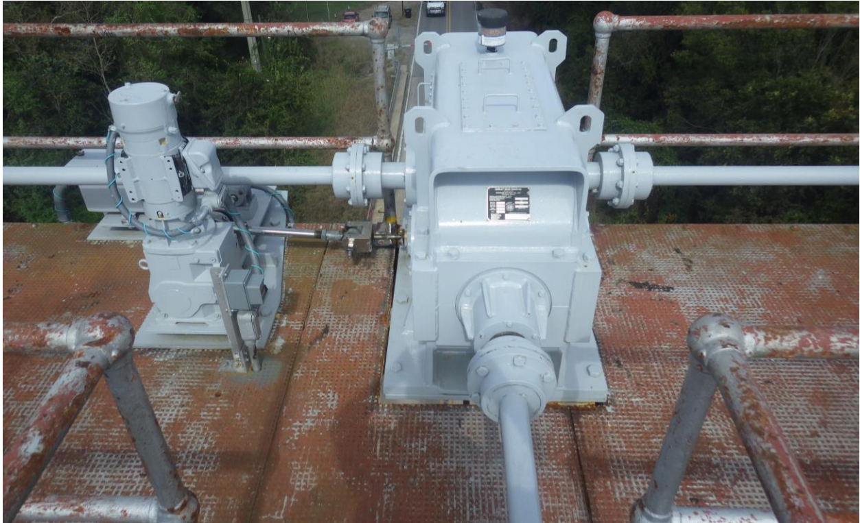
Photo 12 – Lift Span Secondary Reducer with Locking Clutch Assembly
