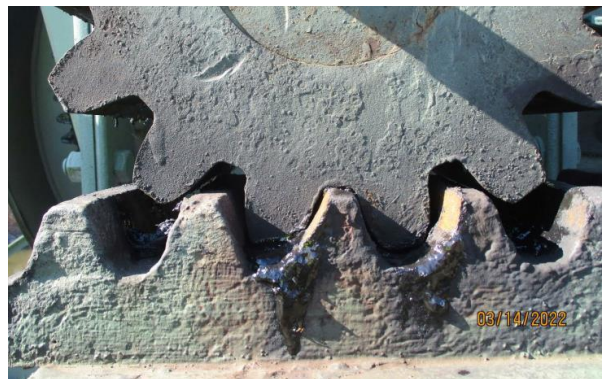
Figure 12: Wear on rack at closed position
