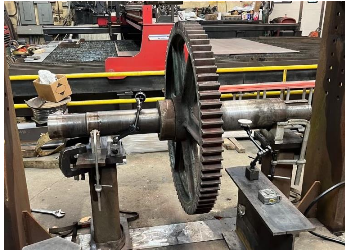
Figure 17: V block setup used in contractors' shop
