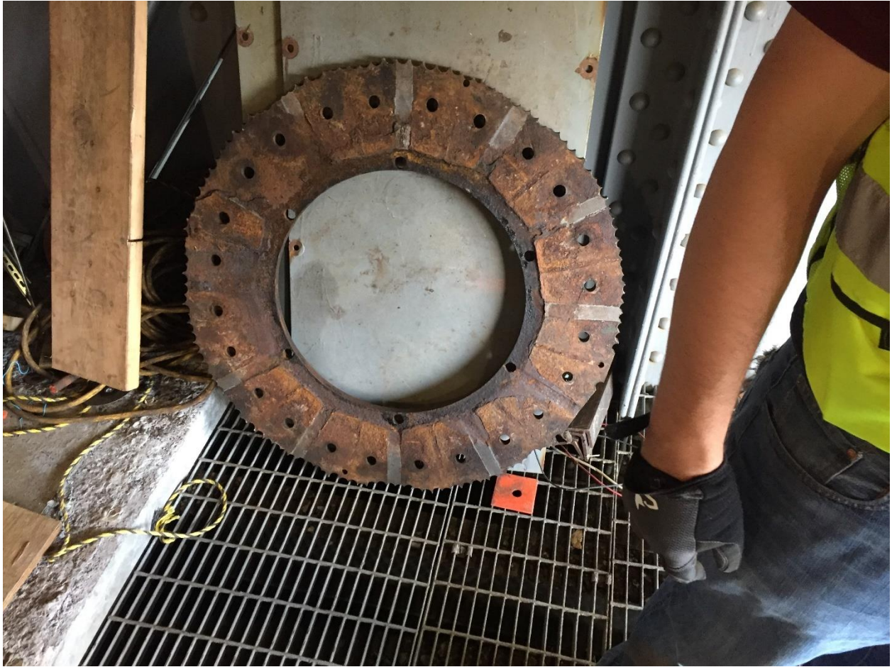
CAPTION: Removed portion of upper gusset plate which was replaced with a temporary plate to limit radial motion during test openings.
