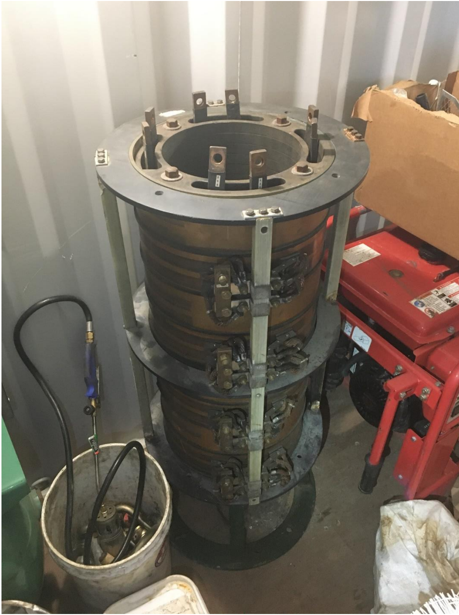
CAPTION: Existing collector ring. Eight rings for 3-phase power from two sources. Instrument drive shaft and control cables pass through the center of the assembly.
