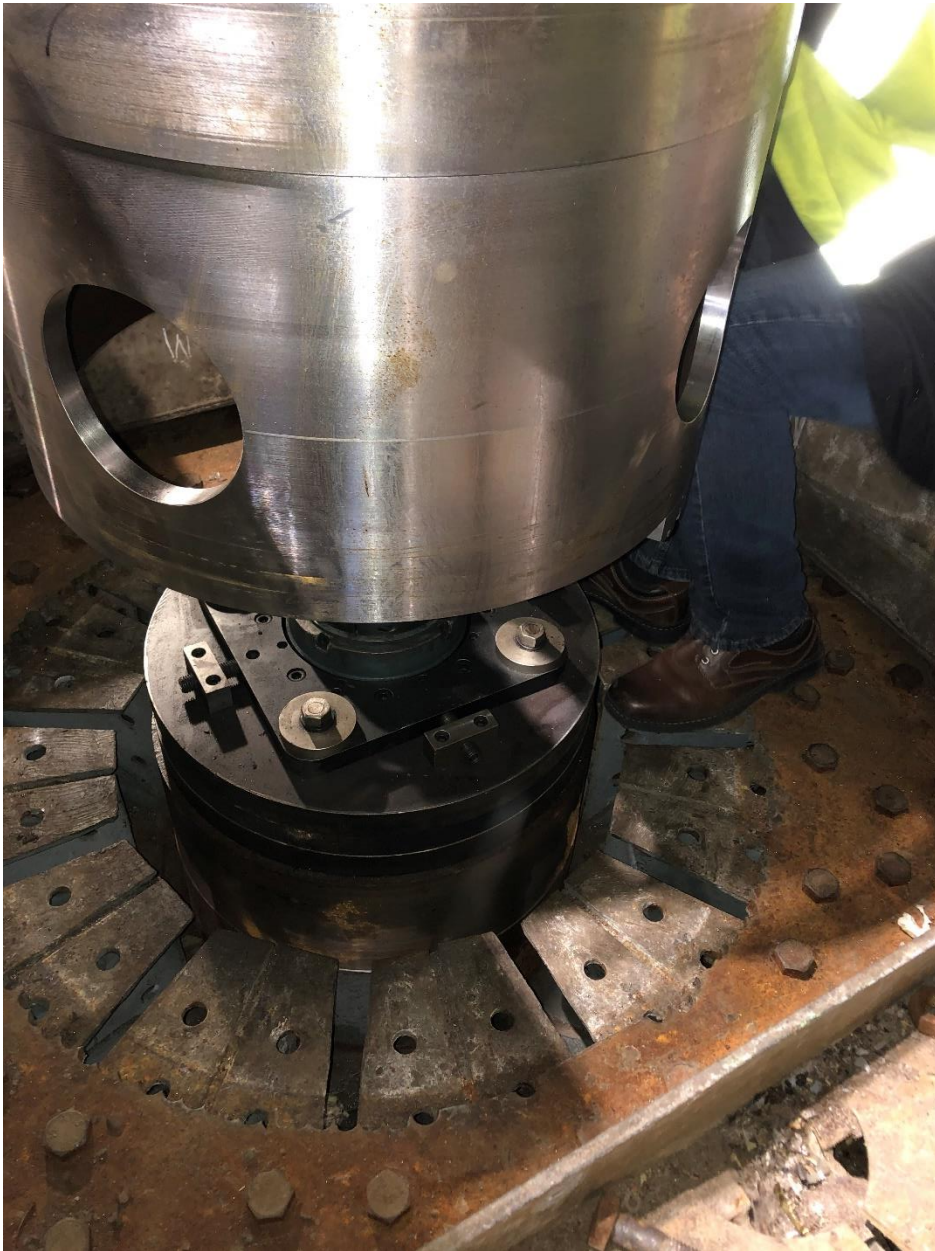
CAPTION: Machining device to machine the cylindrical surface of the center post. The device fits between the post and the ends of the 12 radial struts.
