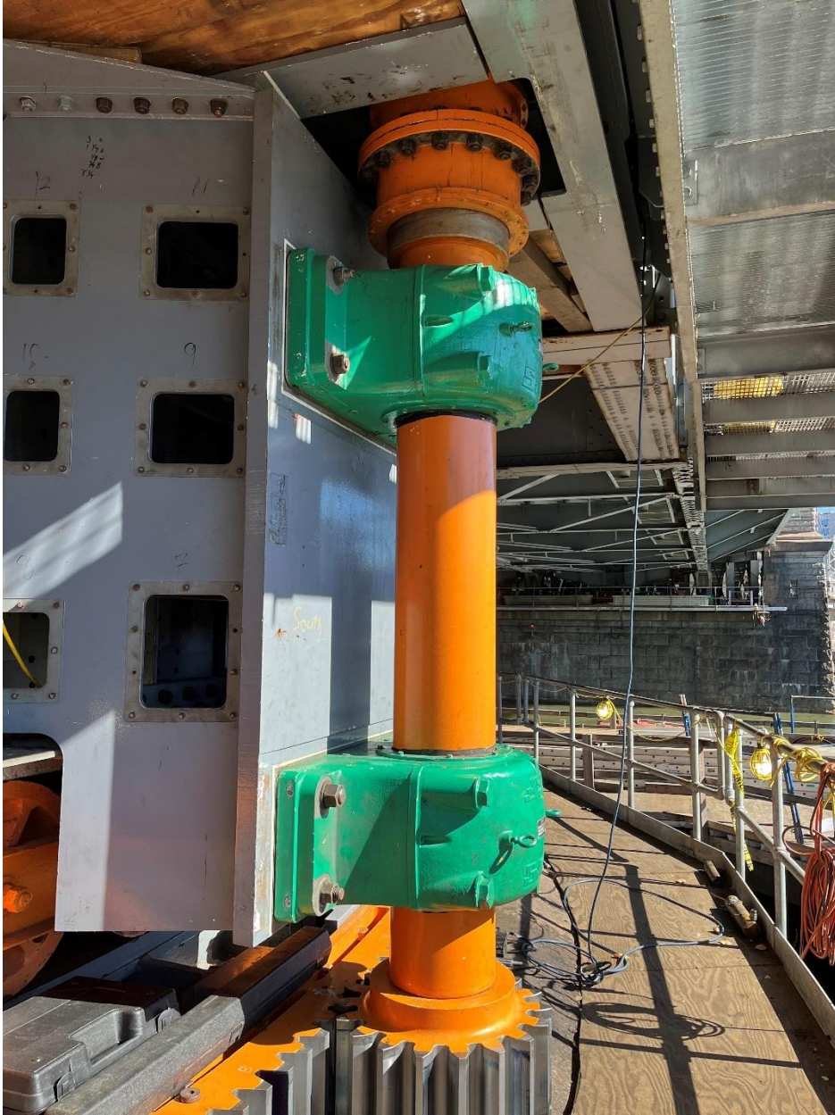
CAPTION: New south pinion in mesh with the rack. Pinion shaft, pillow block bearings, coupling and support are shown.
