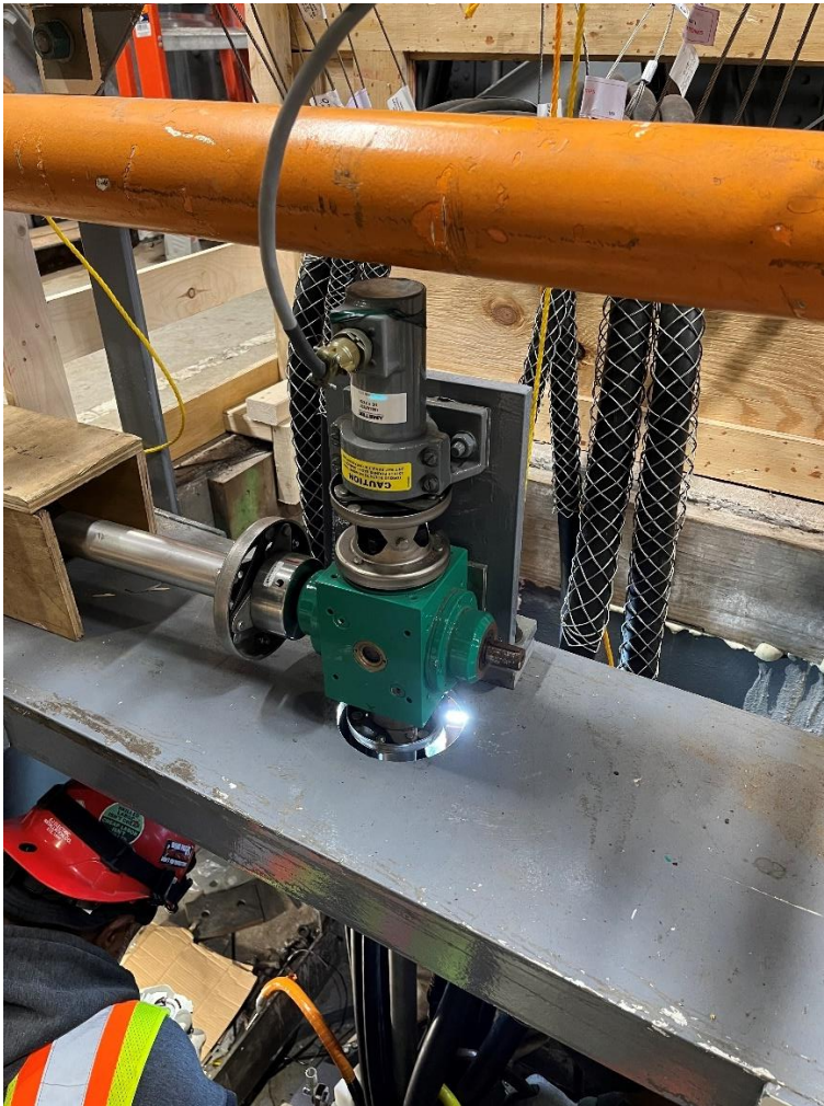
CAPTION: Instrument drive reducer and encoder. The control cables in strain relief fittings pass through the collector ring.
