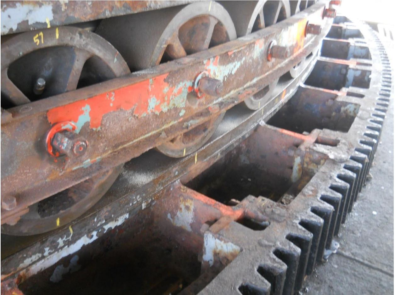
CAPTION: Existing rack, rollers, track chair, upper and lower tracks.
