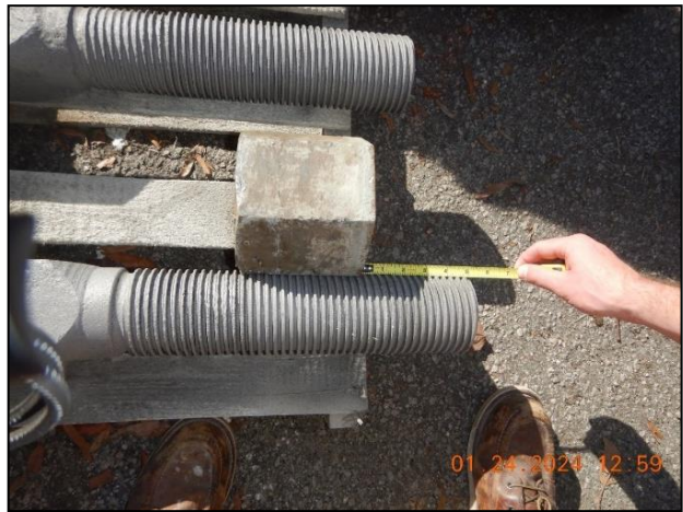
Figure 32: Condition of the existing take-ups following shop cleaning.
