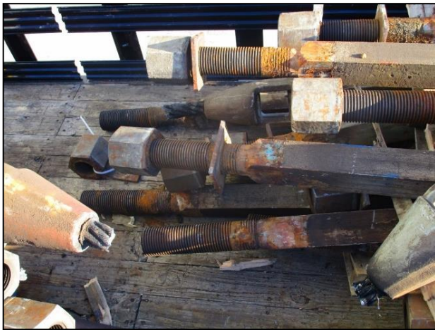
Figure 31: Condition of the existing take-ups removed during the first outage.
