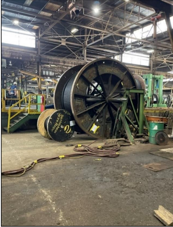
Figure 7: Photo of the wire rope on the spool prior to cutting at Wire Rope Works.
