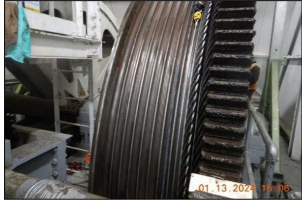
Figure 26: Condition of the wire rope sheaves following cleaning.
