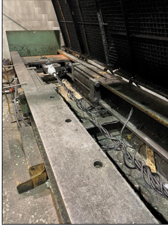
Figure 8: Photo after the break test of the wire rope at Wire Rope Works.
