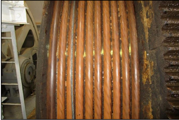
Figure 25: Condition of the wire rope sheaves prior to cleaning.
