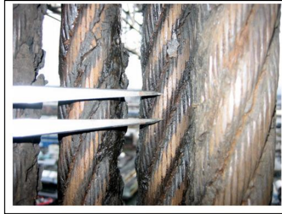
Figure 4: Measurements taken on the outer wires during the 2013 investigation.
