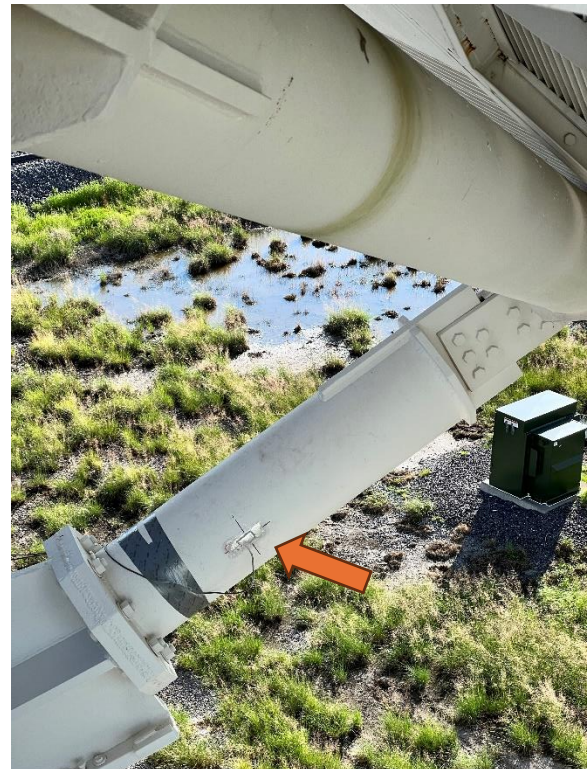
Photo 7 Strain Gage Installed on Dish
