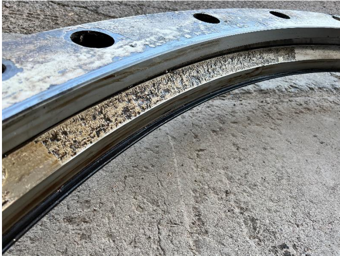
Photo 10 Damage to the Azimuth Bearing Race
