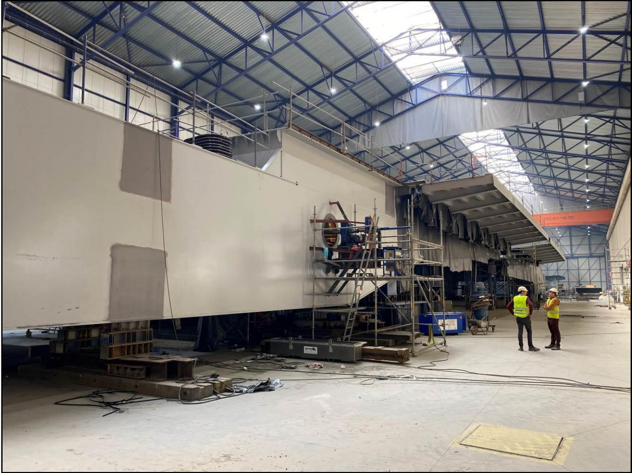
Figure 6 – Bascule Leaves in Fabrication, Each leaf supported in it's final deflected condition for machining of the trunnion bores and other machinery mounting surfaces
