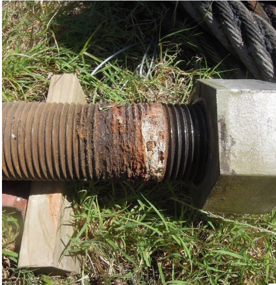
Figure 2: Heavily corroded threads were discovered in the portion of the take-up that passed through the billet.
