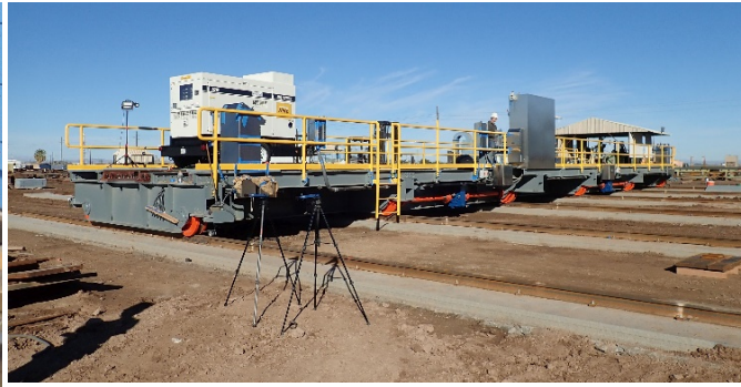
Photograph 13 – Fully assembled transfer table on temporary crane rail track at the shop in El Centro
