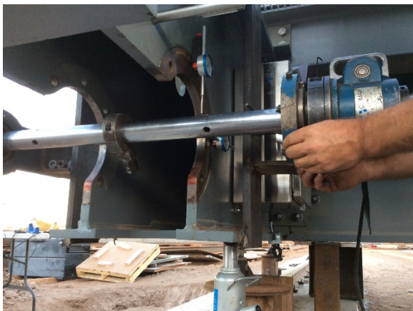
Photograph 11 – Lineboring trucks on fully assembled table for wheel block hubs
