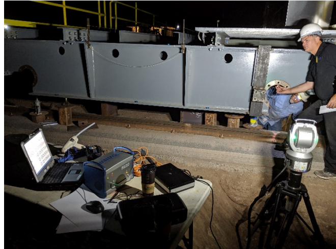
Photograph 10 – FARO laser tracker was used to map wheel block bores
