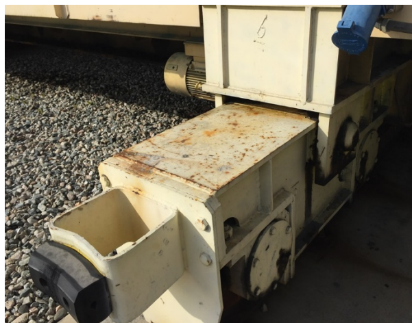
Photograph 4 – Original transfer table drive truck
