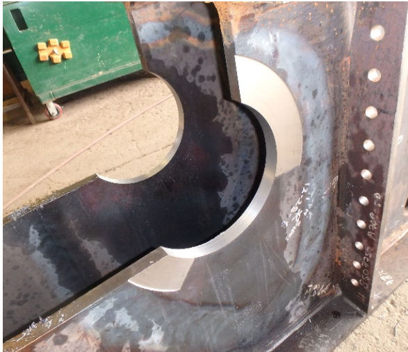
Photograph 9 – Machining warped truck web for wheel block installation
