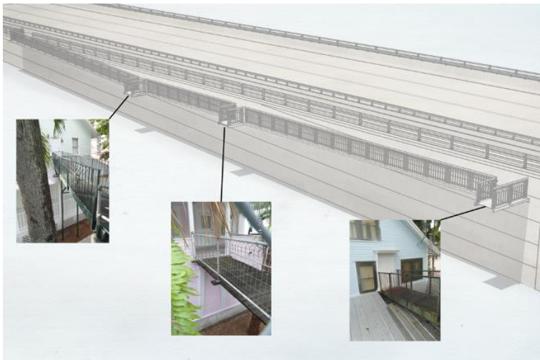
Provision was made to connect to the existing catwalks at the Miami River Inn.
