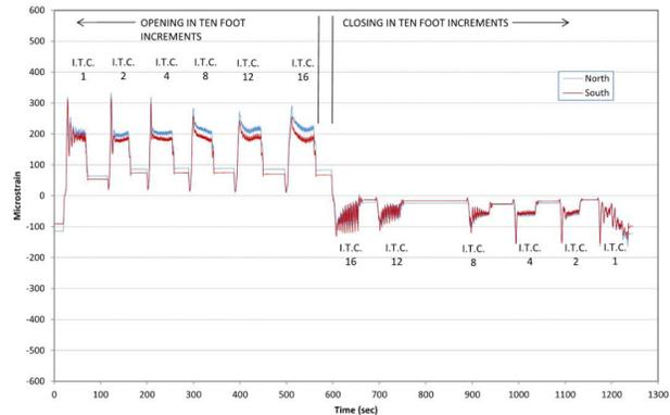
FIGURE 6: Lorain Lift Bridge. Strain Recordings of Integral Time Constant Adjustments at the Drive.
