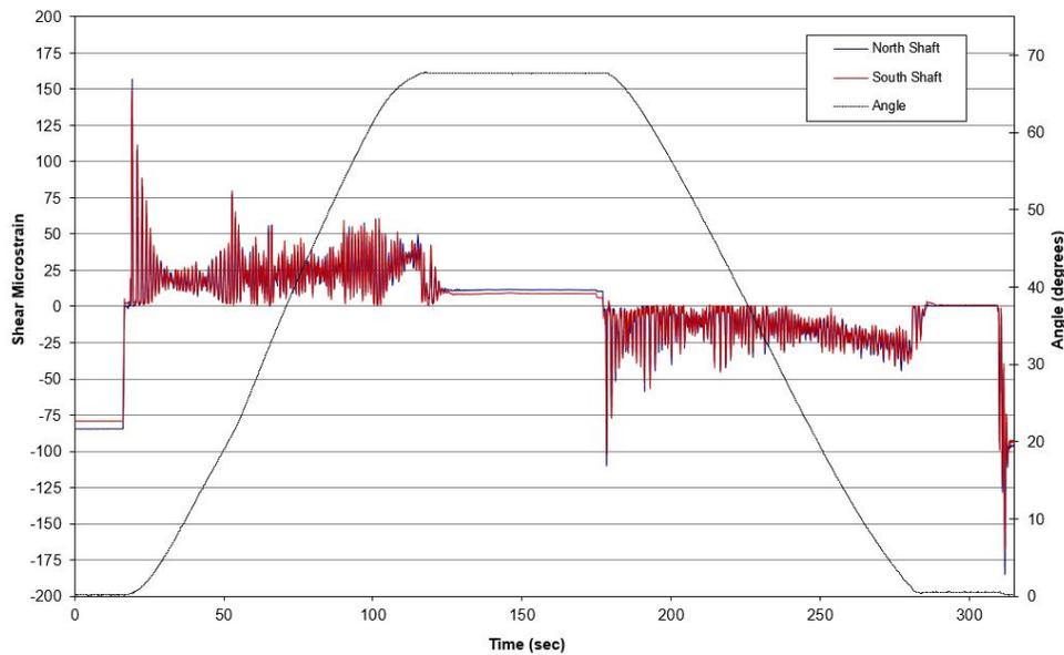
FIGURE 15: LaSalle Causeway Bascule Bridge. Strain Gage Recording After Repairs to the Differential Assembly.
