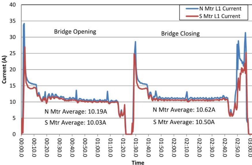
FIGURE 10: Hines Memorial Bridge. Motor Current after Tuning.
