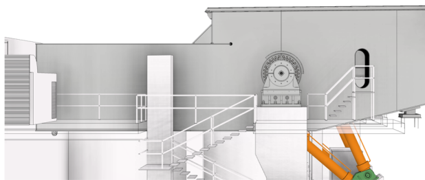
Figure 5: Bascule Girder as Modeled in Inventor
