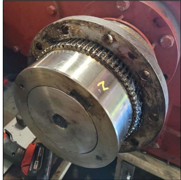
Photo 12: Final Coupling Installation
