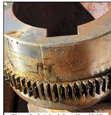
Photo 8: Original Coupling Half After Removal
