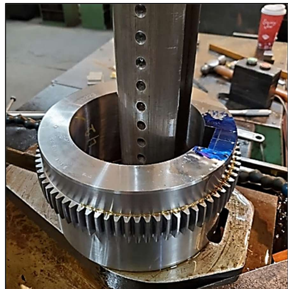
Photo 11: Shop Machining of The Sacrificial Coupling Keyway
