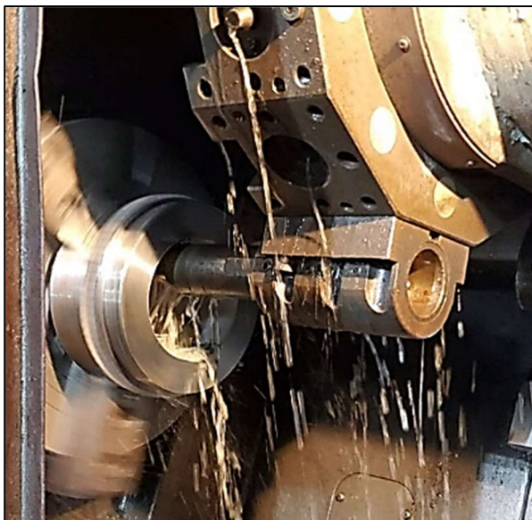
Photo 10: Shop Machining of The Sacrificial Coupling Bore
