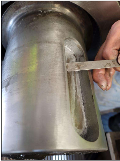
Photo 9: Existing Shaft Keyway Measurements
