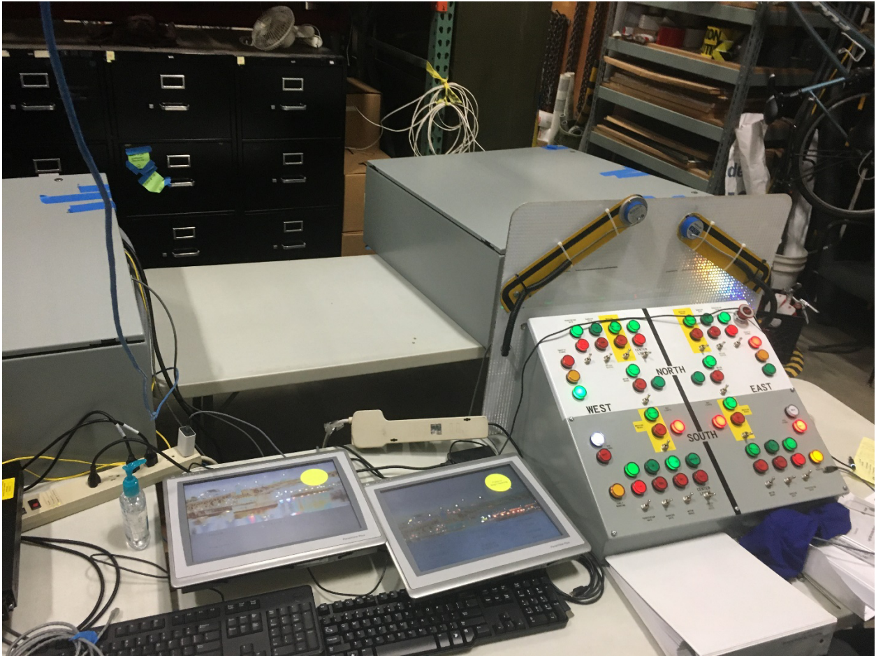
Figure 7 Emulation switch board, HMI touch screens, usb keyboards for touchscreen configuration input. In the background are a pair of plc systems in enclosures with drive communications ethernet cables tied to the post.
