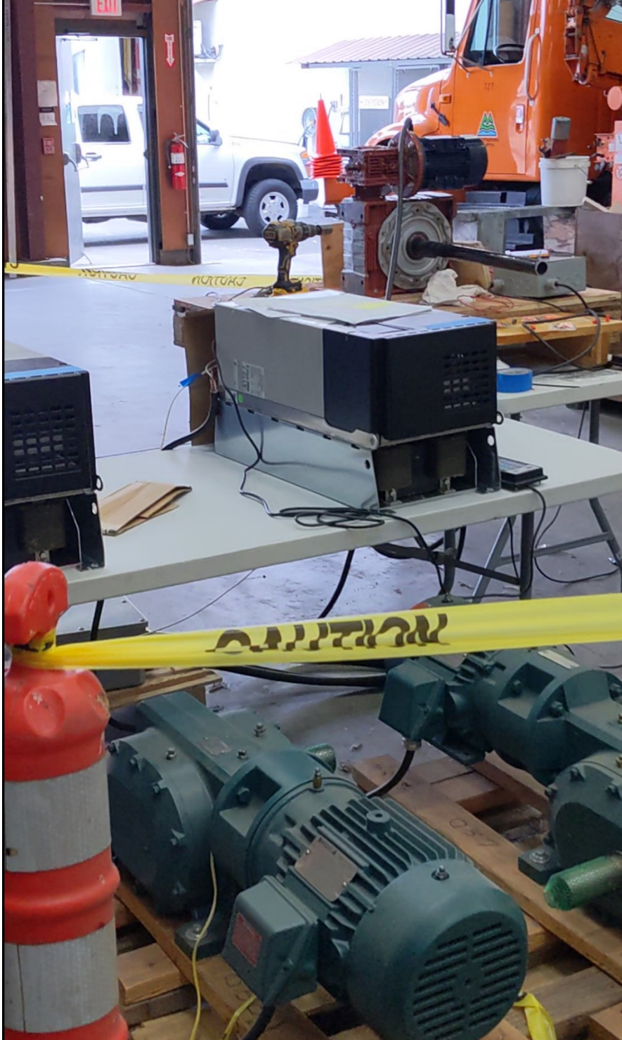
Figure 8 480V ac powered new motor drives at bridge shop, connected to gearbox motors in foreground for motor control testing of speed and rotation direction commands. Encoder setup and motor control testing was performed on the red gear motor system in the background used for the Broadway Bridge streetcar 600V overhead catenary disconnect system.
