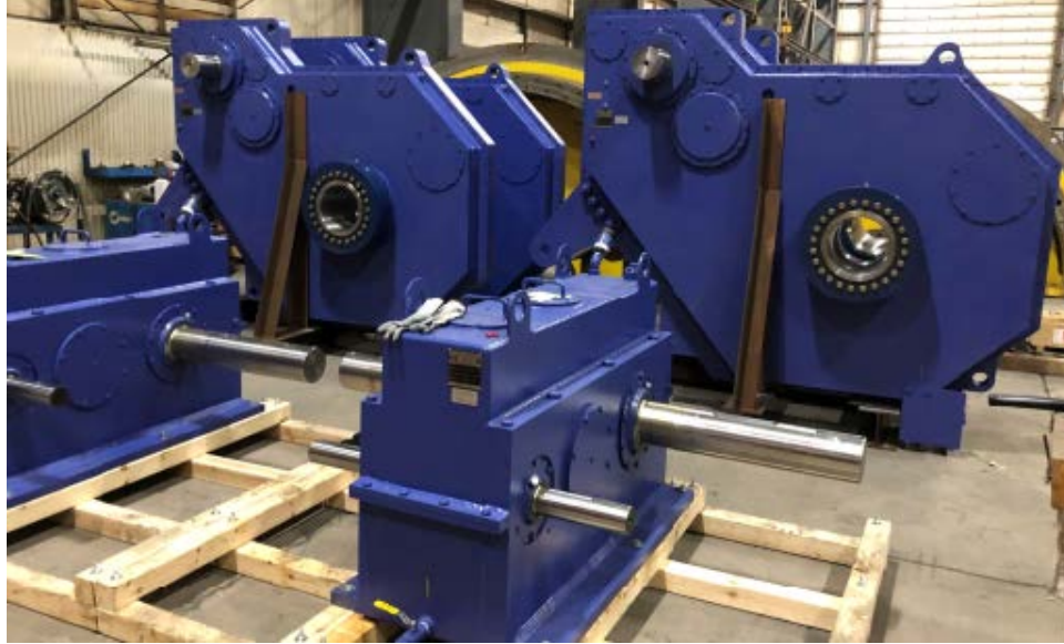
Enclosed Gearboxes – in long term storage
