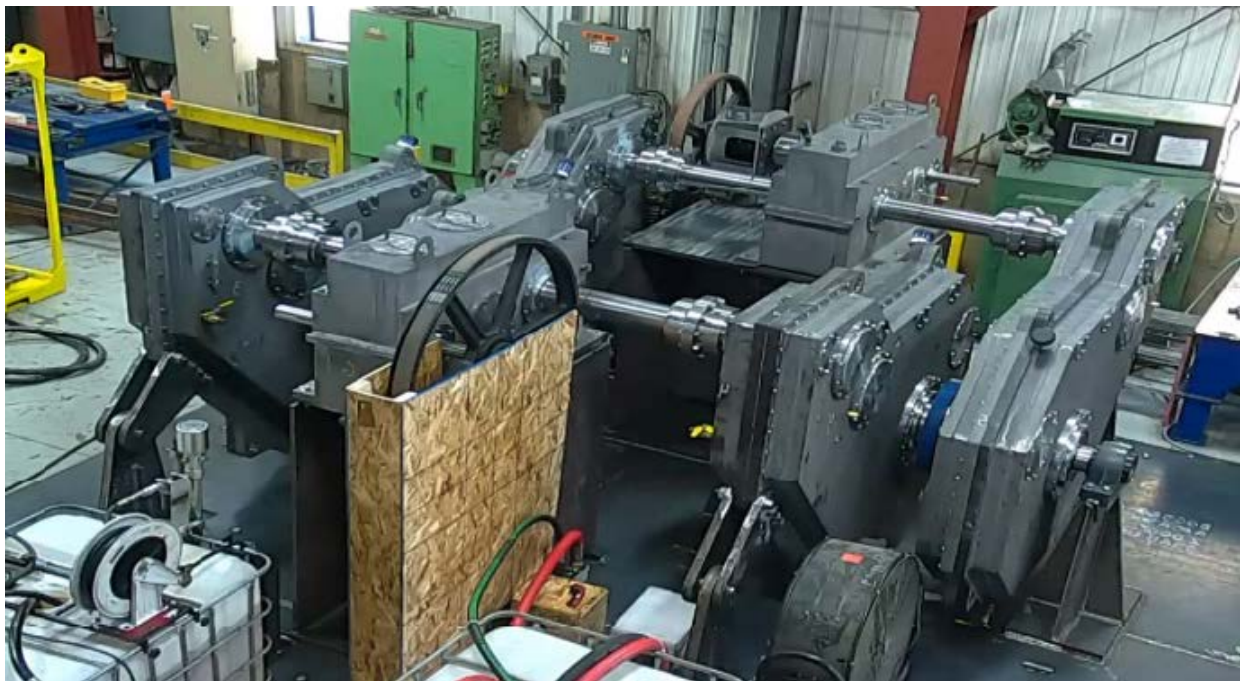
Enclosed Gearbox Factory Acceptance Testing with the units connected in tandem Dynamic tests witnessed remotely via video conference
