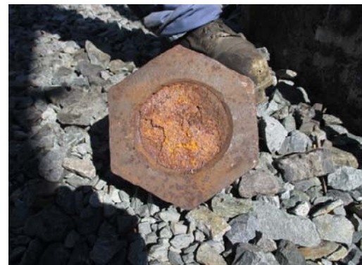
Figure 7 – Failed Bolt. As found at siding. The workman's boot behind the nut at top provides a reference for size.
