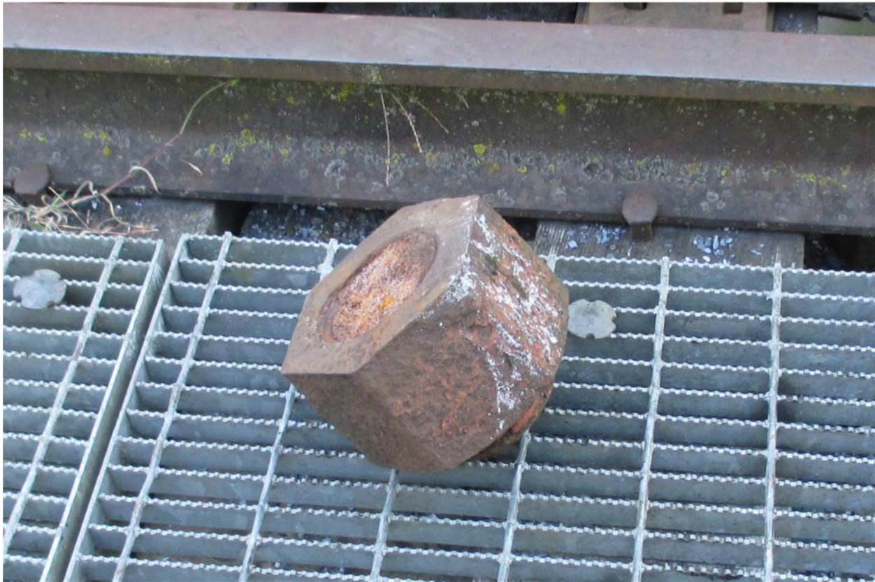
Figure 1 - View of failed end of 4 \frac{3}{4} " diameter bolt. Bolt is resting on standard walking grating adjacent to track for reference of size.
