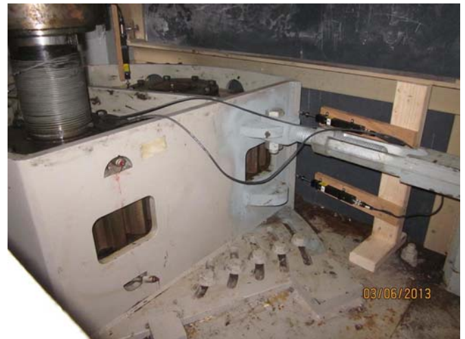
Figure 6. Lower Gear Box Assembly. The assembly is shown with instrumentation for LVDT deflection measurements and strain recordings at the pinion shaft.
