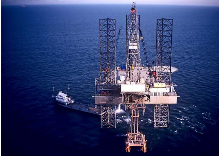
Three-Legged (Truss Leg) Lift Boat built for drilling and maintaining oil wells.
