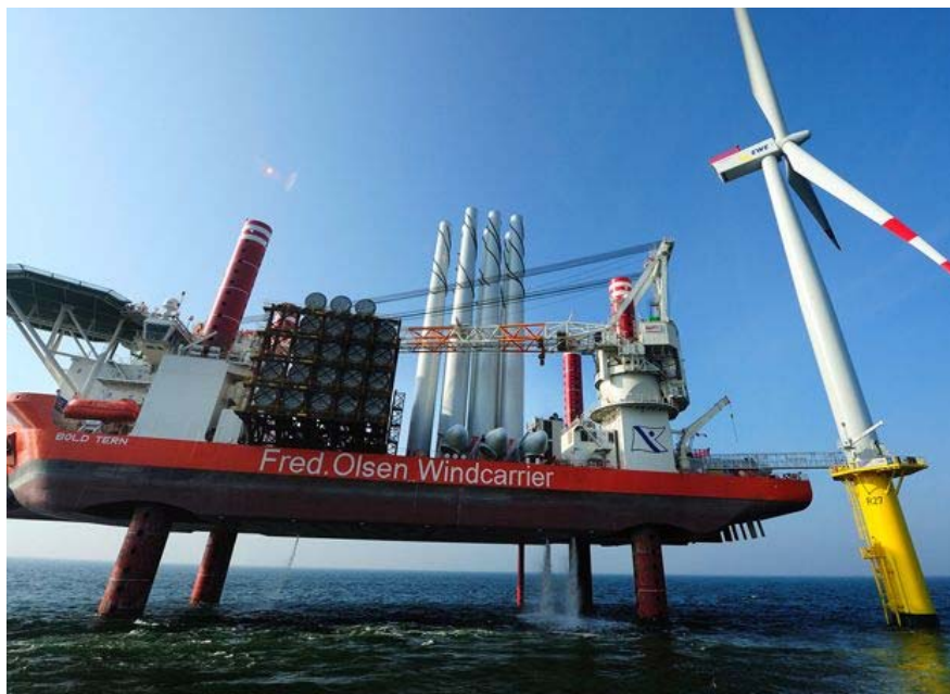
Four-Legged (Pipe Leg) Lift Boat built for Wind Turbine Maintenance
