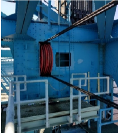
FIGURE 7: Operating Ropes Through Deflector Sheave
