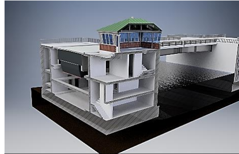
Section through Pier and Control House of Proposed New North Hero Bridge
