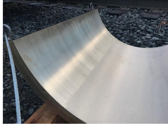
Photo 18: Close up view of the relief added to the counterweight side of the trunnion bearing bushing.
