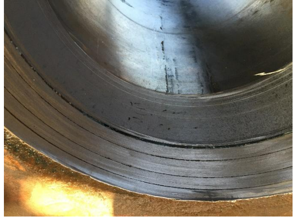
Photo 36: Close up view of truss and sleeve after line boring.
