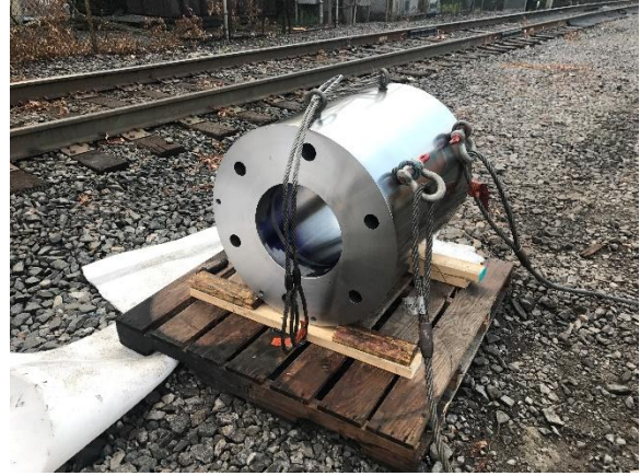
Photo 30: The new sleeve finish machined except for the inside diameter and ready for installation.
