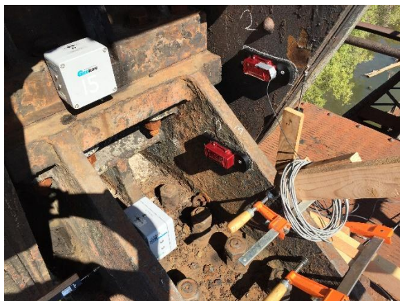
Photo 11: Instrumentation installed on the counterweight trunnion bearing
