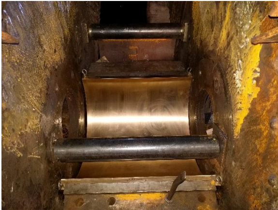
Photo 31: The new bushing after installation in the existing bearing housing.
