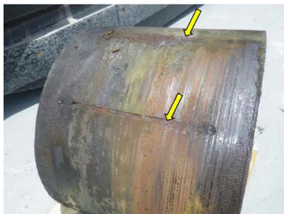
Photograph 5 - Lakeside 2 nd Link main sleeve with grease grooves packed with solidified grease
