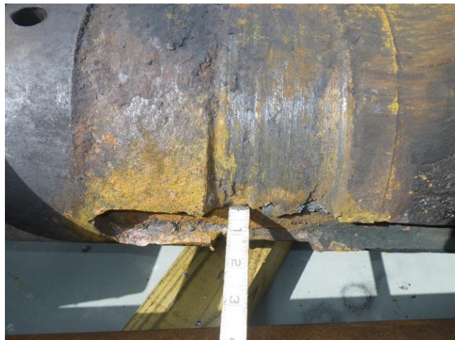
Photograph 6 - Lakeside 2 nd Link Pin with wear steps up to 1/2" deep and severe abrasion
