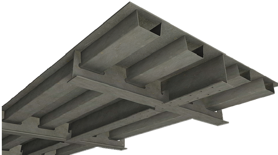
Figure 2: Typical orthotropic deck section
