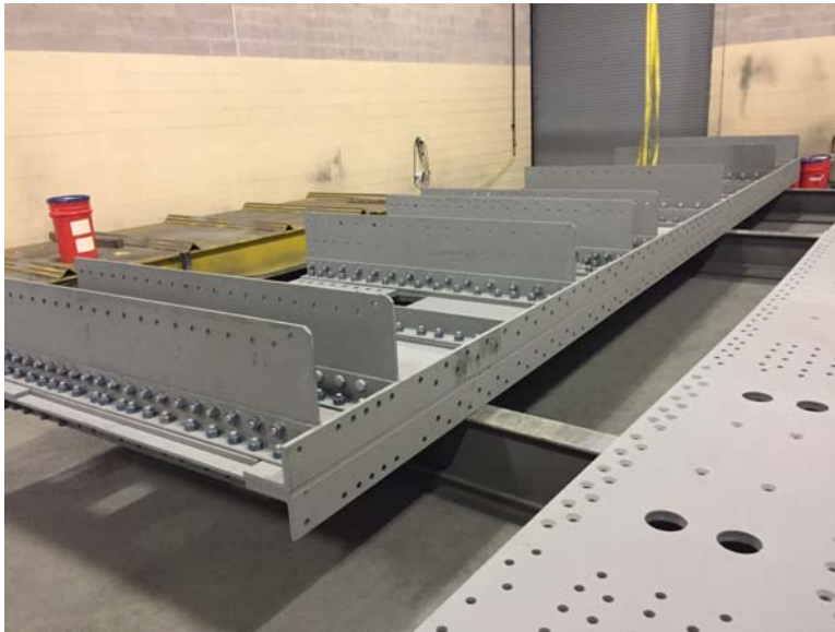
Figure 7: New Longitudinal Girder in Fabrication
