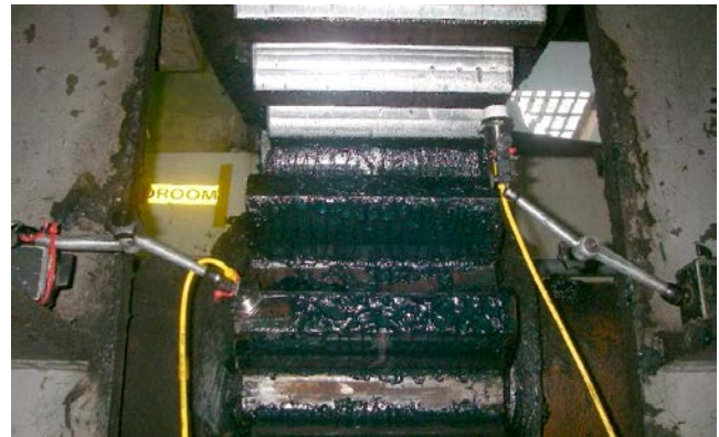
Photograph 5 – Measuring gear runout during operation with inductive non-contact distance sensors
