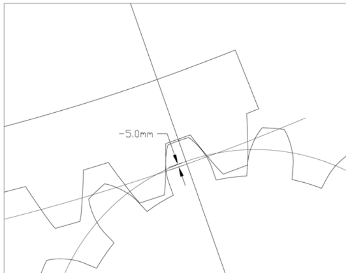
Figure 6 – Scale drawing of rack/pinion mesh over-engaged 0.200" (5mm)
