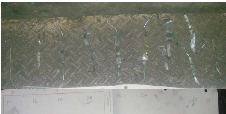
Photograph 7 – Flattened lead solder after operation
