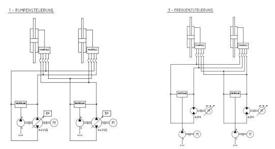
The Question is of course which one to use. From the electric point of view, it makes sense to change the speed of the E-motor to control the pump flow. From the hydraulic point of view it makes sense to control the flow by means of a constant speed E-motor in combination with variable pump. From the service point of view, for both the solutions pros and cons can be stated.
