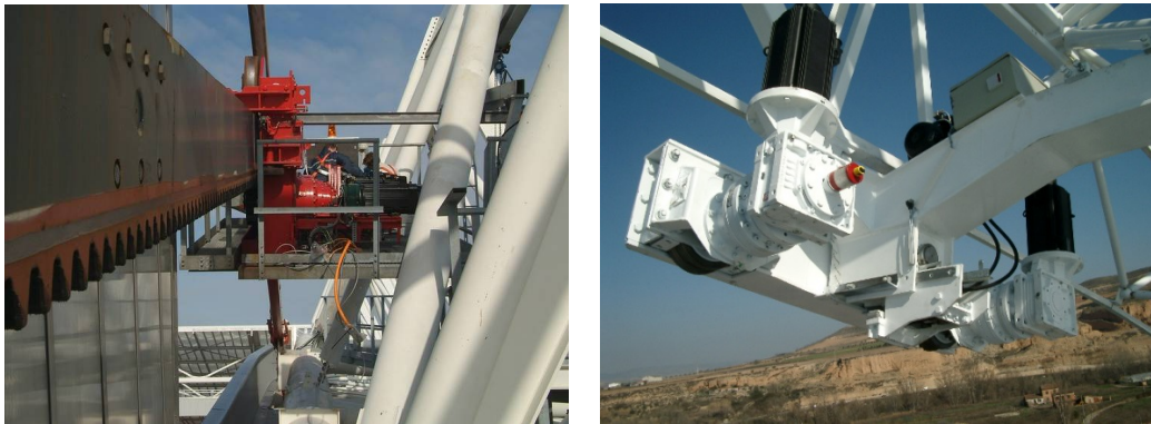
Figure 8: Rack and pinion drive unit (Amsterdam Arena left, Plaza de Illumbre, Spain, right) [17]
