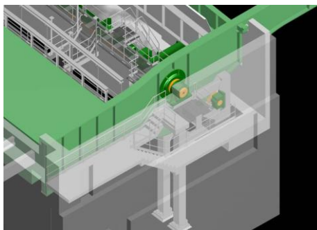
Fig. 1: Bascule Span Pier and Machinery Room
