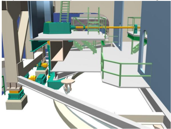
Fig. 6: Swing Span Bridge Pivot Pier Coordination
