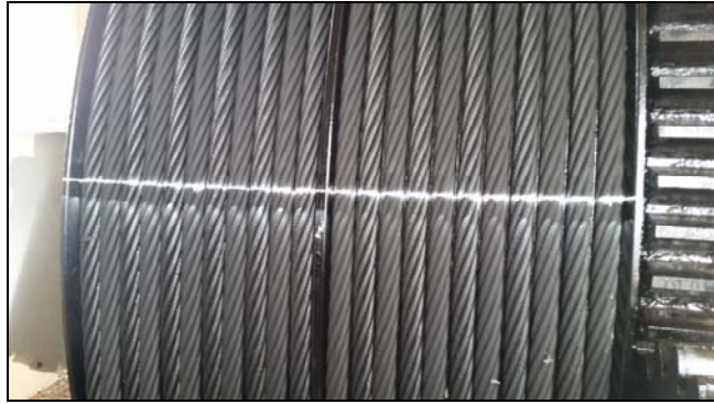
Figure 9. A painted line is used to monitor rope slippage at this counterweight sheave.
