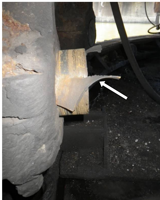
Figure 4. East balance wheel shaft bushing deterioration from excessive loading conditions.
