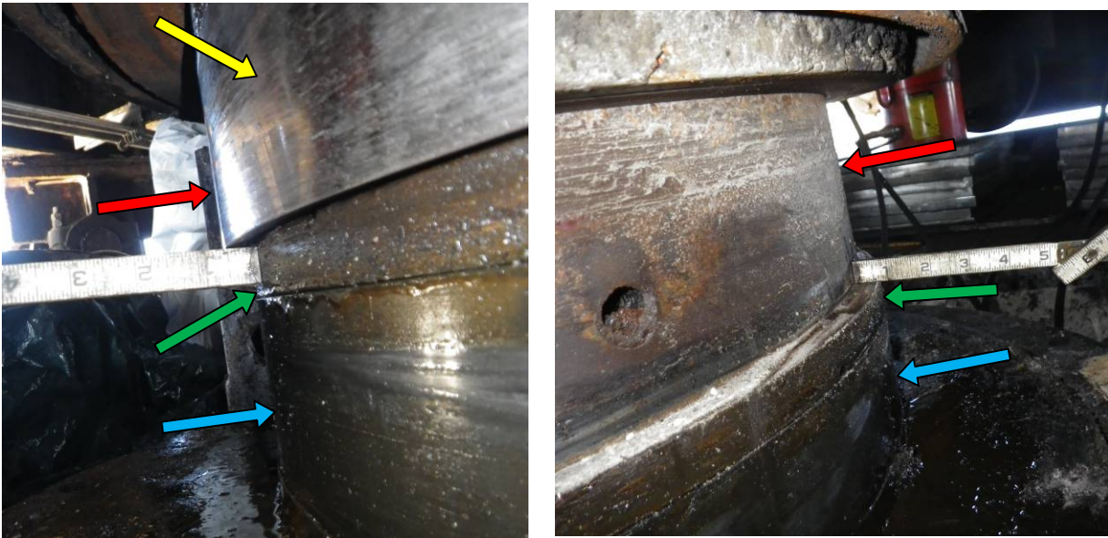
Figure 10. Opposite sides of the pivot bearing showing the \frac{1}{2} " displaced position of the top steel disc (red arrow) relative to the bronze disc (green arrow) and bottom steel disc (blue arrow) discovered once the oil box was removed. Note signs of hard contact with the oil box on the top steel disc (yellow arrow)
