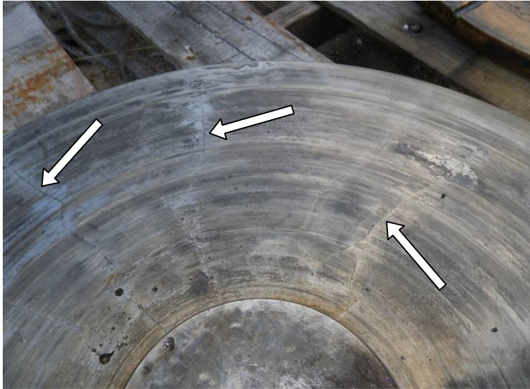
Figure 11. Bottom surface of the existing bottom steel disc with several significant cracks and signs of wear at the lower casting interface.
