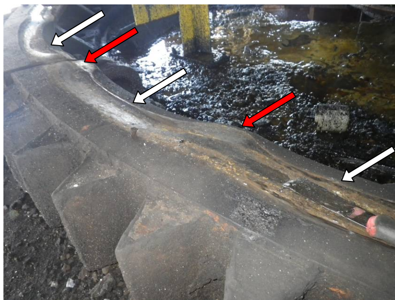
Figure 5. Severe wear and plastic deformation of the east balance wheel track from excessive loading conditions. Note peaks (red arrows) and valleys (white arrows)
