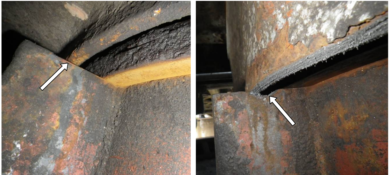
Figure 8. Change in unintended contact and wear between the east side of the upper casting and the oil box over a period of a year and a half.
