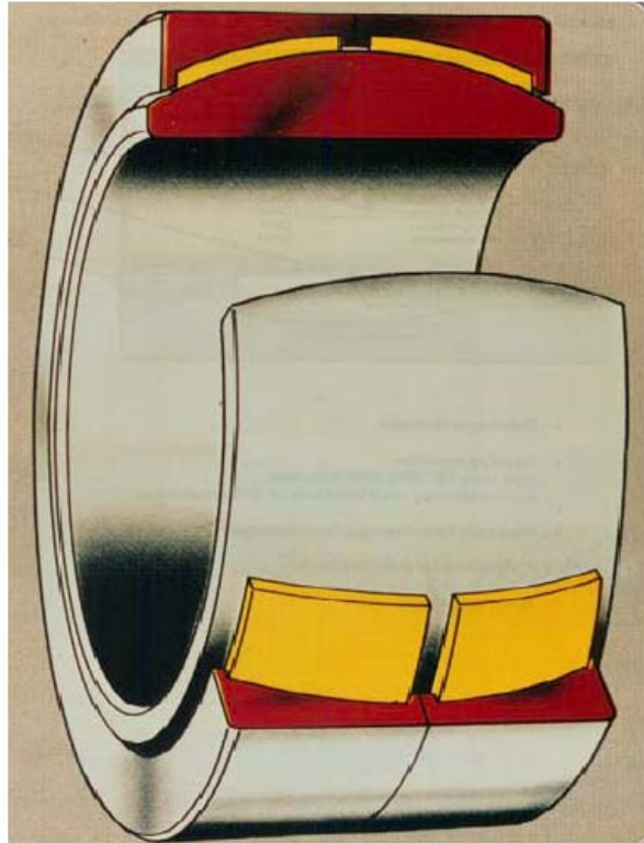
Figure 11 – Drawing of Spherical Plain Bearing used on Erasmus Bridge
