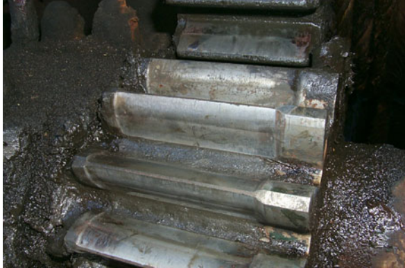
Figure 4: Operating Drum Pinion. Note severe tooth wear.
