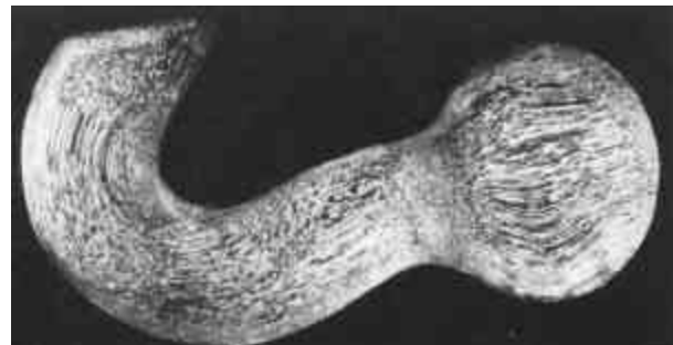
Fig. 3 Forging Flow in a Crane Hook
