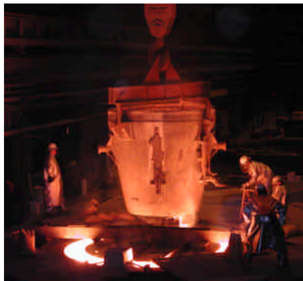
Fig. 1 Bottom Pouring in a Steel Foundry
