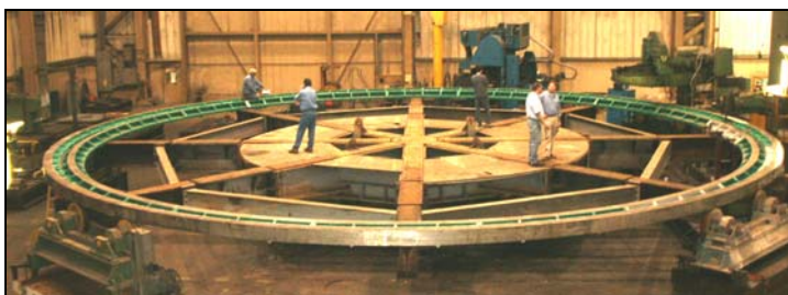
PHOTO 5: Machining of Rack and Track in Shop
