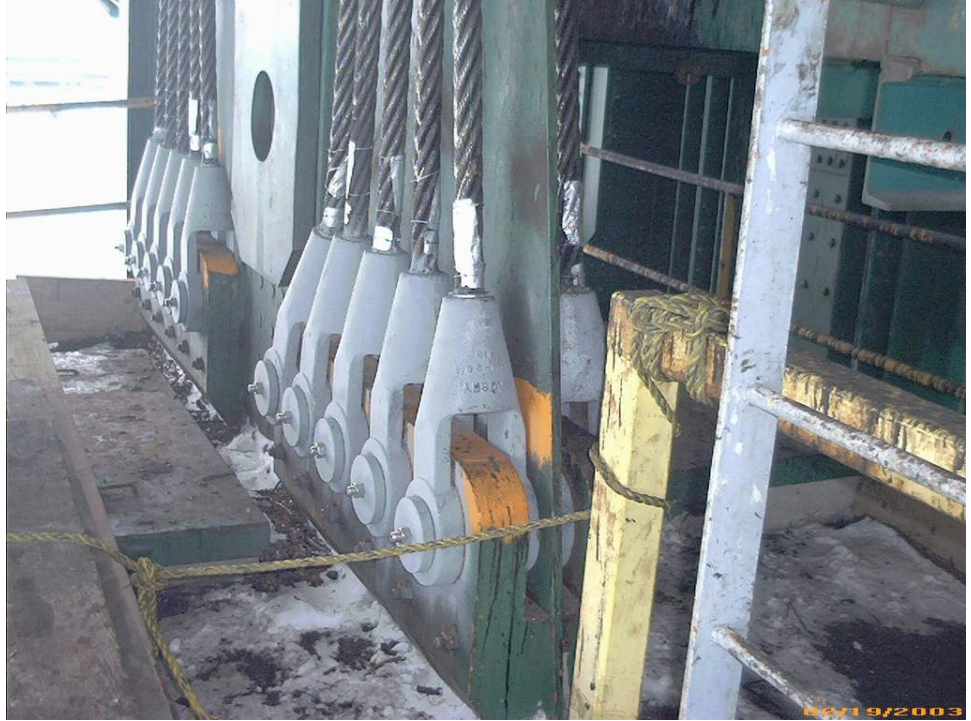
New Ropes Attached at Counterweight
