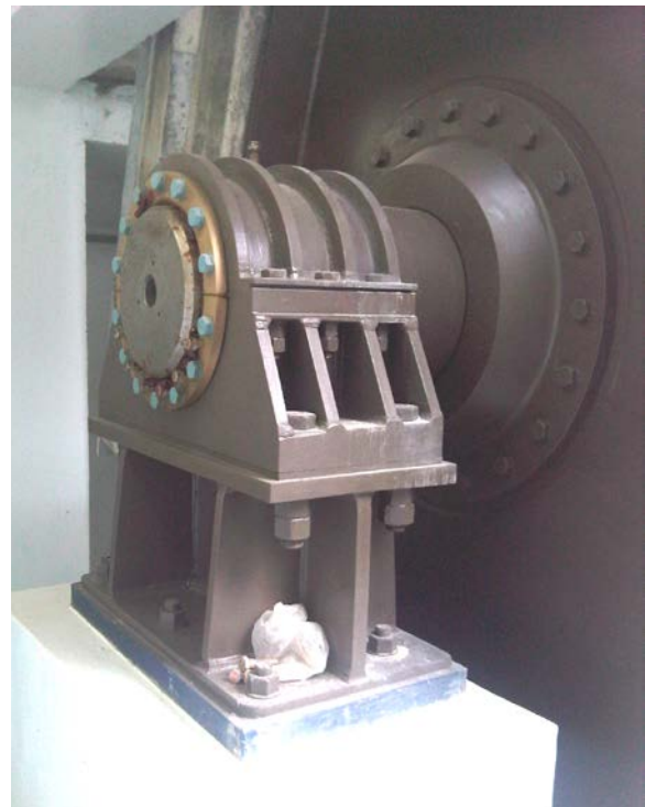
Typical Trunnion / Plain Trunnion Bearing Assembly – Port Ferdinand Bridge, Barbados, West Indies
