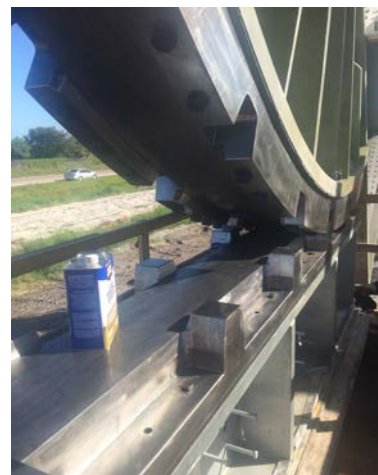
Photograph of Tread (upper) with Pockets and Track (lower) with Lugs
