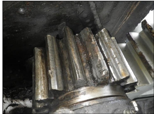
Photograph 13 - Existing condition of West G3 pinion with new G2 gear
