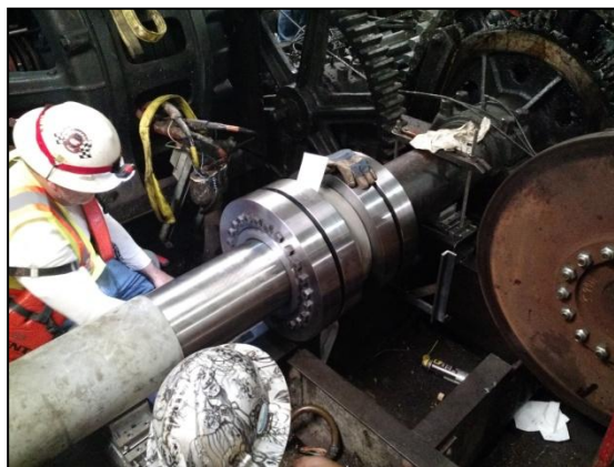
Photograph 21 - Sleeve coupling with Tollok shrink discs installed
