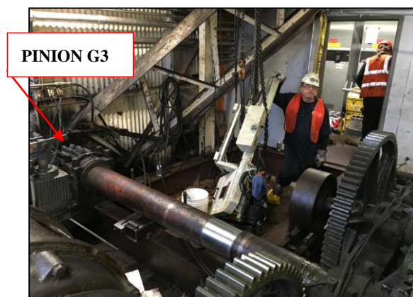
Photograph 15 - Structural bracing members above G3 pinion impede removal
