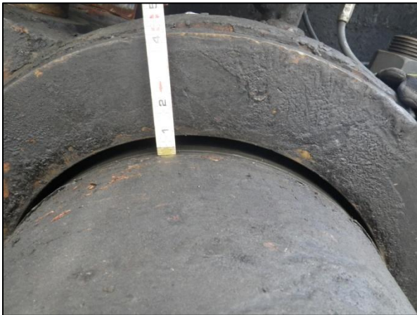
Photograph 3 - Excessive clearance at West Bearing B1
