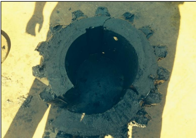
Photograph 12 - View of the damaged pinion gear that was removed from the East drive shaft.
