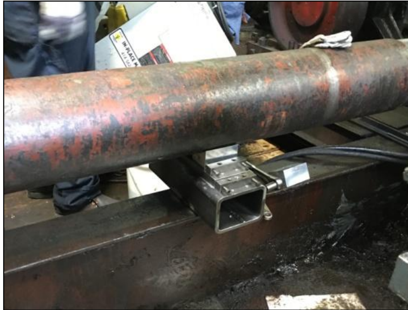
Photograph 16 - Adjustable V-block to support shaft and align the cross shafts
