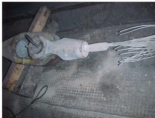
Photo #9, Tensile test of sample # 5
