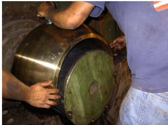
Photo – New Bushing Installation
