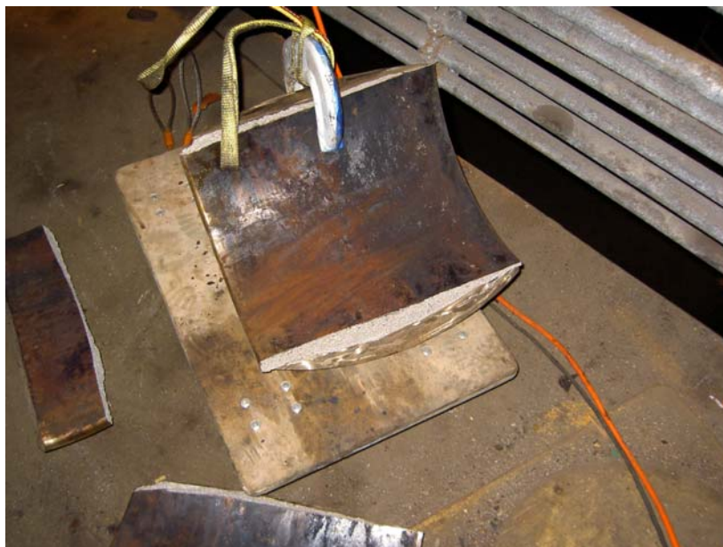
Photo – Trimmed Bushing
