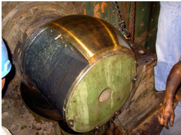
Photo – New Bushing Assembly
