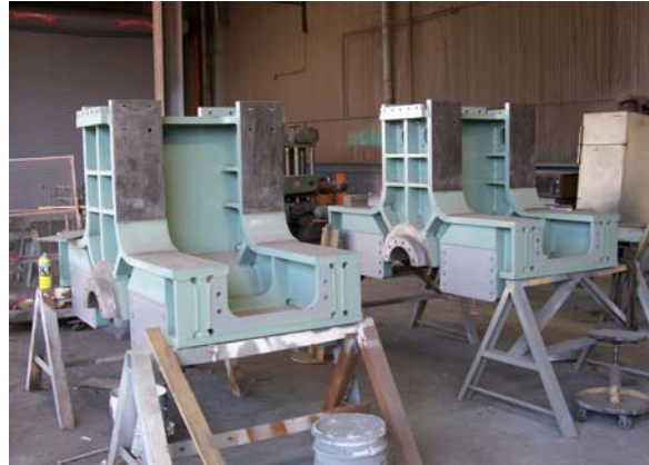
Photo 4: Idler Truck Frames shown on work horses during painting.
