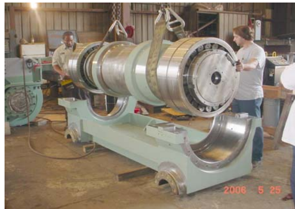
Photo 6: Equalizer Frame and Roller Spindle shown during shop assembly.
