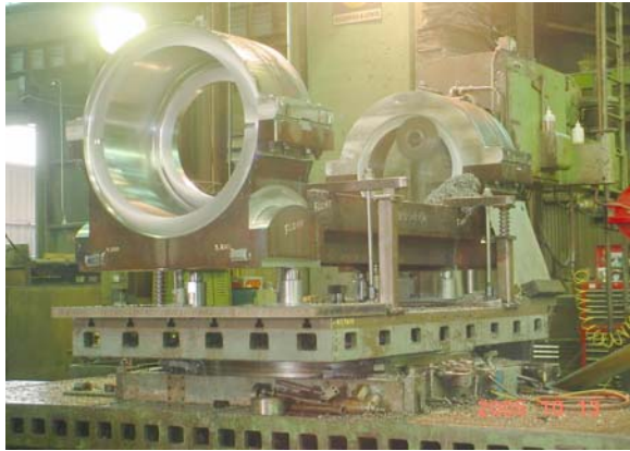
Photo 5: Equalizer Frame shown with Exp. Brg. Housing being reverse counter-bored.
