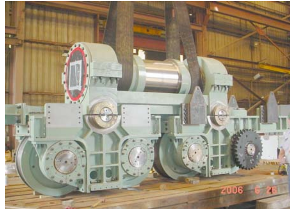
Photo 8: Expansion Assembly shown seated onto Truck Assemblies at shop.
