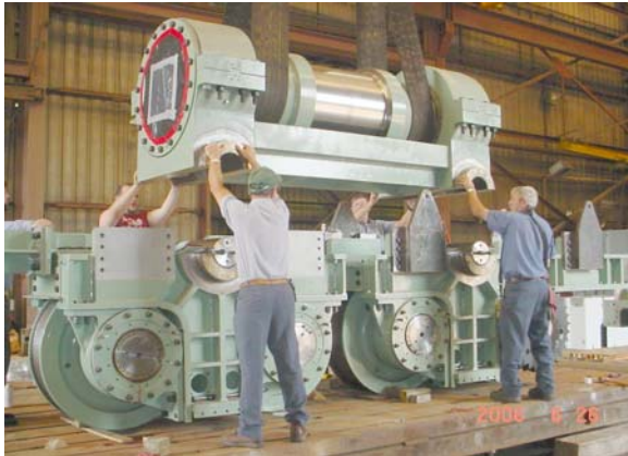
Photo 7: Expansion Assembly shown being lowered onto Truck Assemblies at shop.
