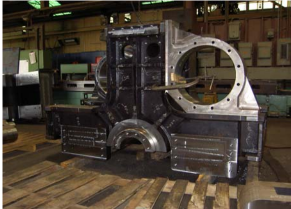
Photo 3: Idler Truck Frame shown after machining with Wheel Bearing Housings.
