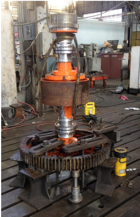
Gear Assembly Prepped for Jacking
