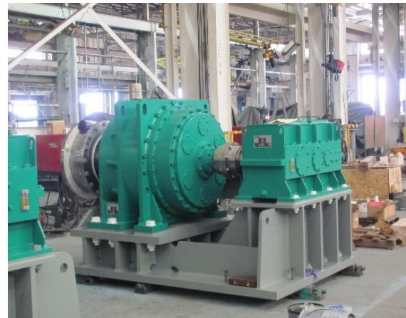
Figure 14: Span Drive Machinery Secondary and primary reducers connected with gear couplings during shop testing.
