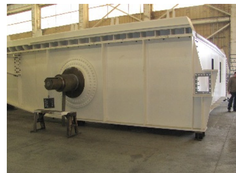
Figure 9: View of the counterweight section of the bascule girder with cantilever Trunnion Shaft and hole for the Tail Lock Receiving Socket
