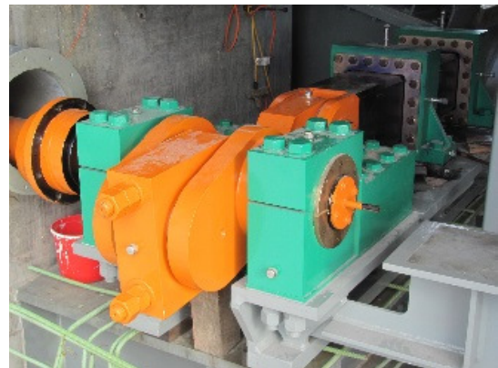
Figure 10: Tail Lock Connecting Rod, Crankshaft and bearings
