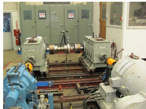
Figure 15: Tail Lock gear reducer testing with output shafts coupled together.
