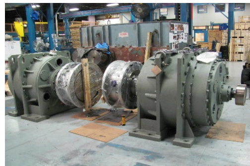
Figure 16: Planetary gear reducers ready for shipment after testing.
