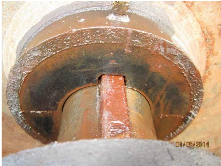
Figure 5 - Gear hub fit with the shaft with excessive clearance.
