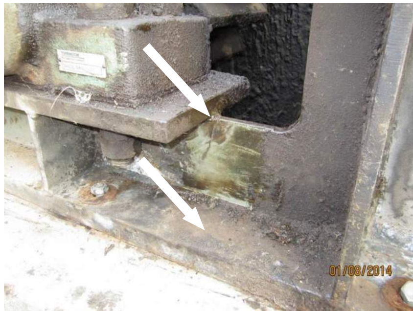
Figure 9 – Different open gear frame with a crack 2/3 the height of the web.
