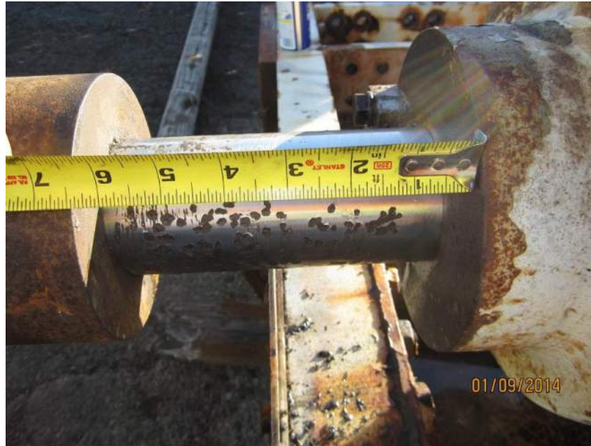
Figure 10 – Air buffer piston rod damaged due to corrosion.
