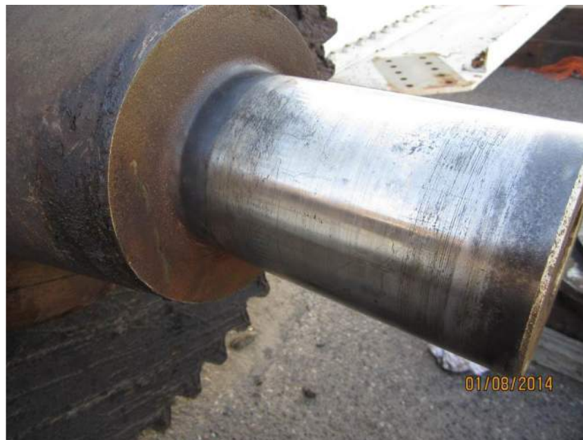
Figure 7 – Bearing journal with moderate scoring and corrosive pitting in the fillet at the shoulder.
