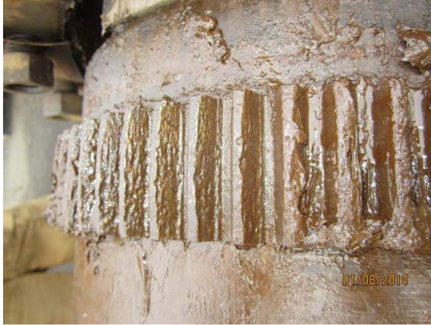
Figure 4 - Gear coupling teeth severely damaged due to corrosion.
