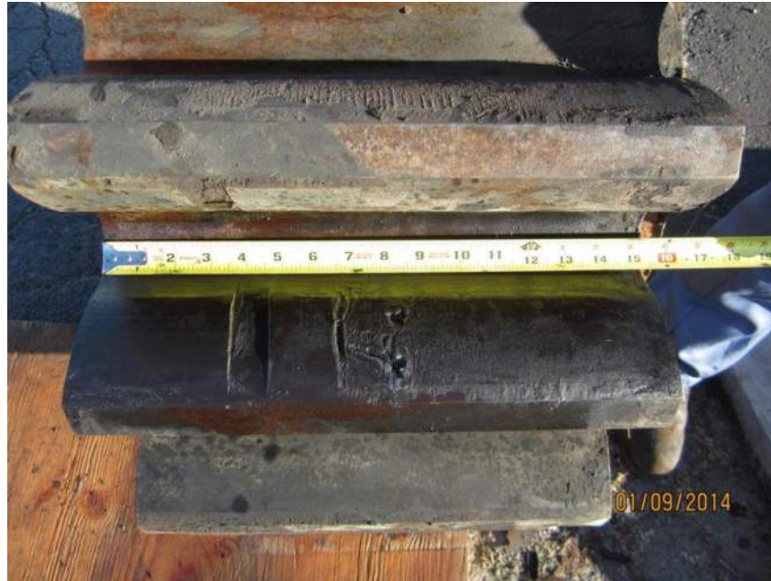
Figure 6 - Gear teeth with isolated damage.
