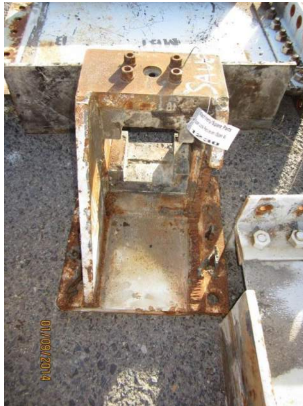
Figure 12 – Both span lock front guides were badly damaged and were replaced. Shoes were salvaged.
