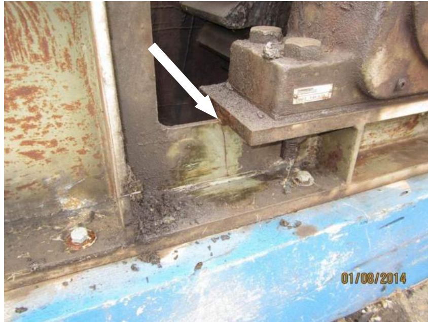
Figure 8 – Open gear frame with a crack the full height of the web.
