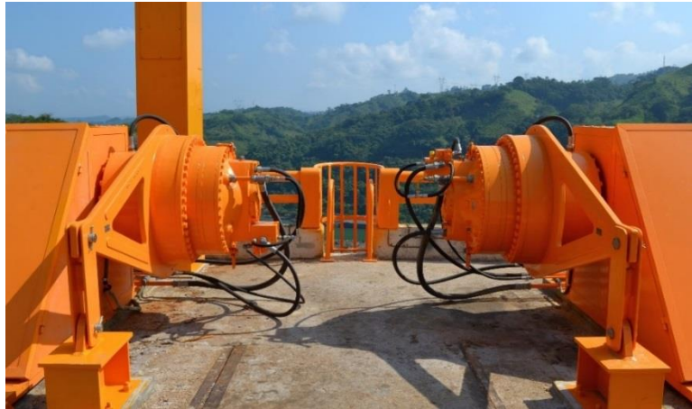
figure 4: direct hydraulic drive
