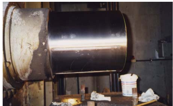
PHOTO4: Trunnion journal for Wappoo Creek Bridge after completion of machining
