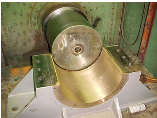
PHOTO 8: Completed Trunnion and Bearing for Wrightsville Beach prior to assembly.
