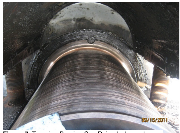
Figure 7. Trunnion Bearing Cap Raised. Journal exhibits severe abrasive scoring along entire length.
