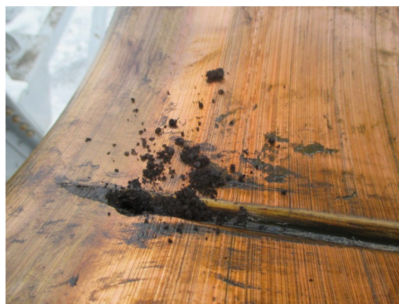
Figure 9. View of hardened grease that has been forcibly removed from the grease port at bottom dead center of the bushing.
