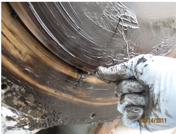
Figure 6. Metal Shavings pulled from Trunnion Bearing Grease Groove.
