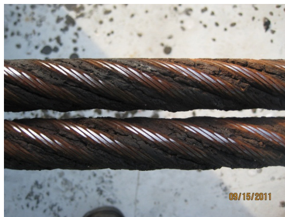
Figure 2. View of wear flats on crowns of operating ropes.
