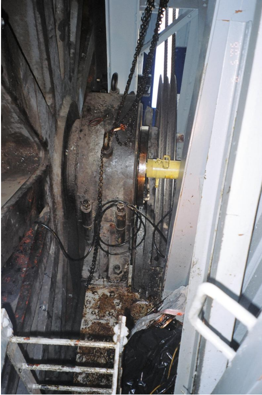
Photo 4: Push Plate and Jack Assembly
