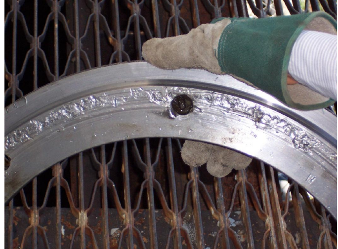
Photo 2: Southern Most Outboard Lock Plate Note severe damage to mounting face.
