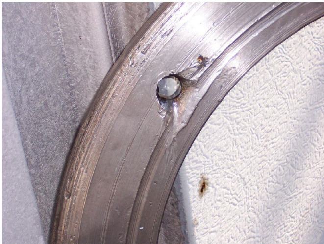
Photo 1: Southern Most Outboard Lock Plate. Note severe damage to hole and outside edge.
